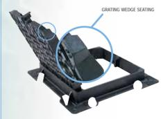
The concept works by converting the downwardforces applied by vehicular traffic into horizontal forces. These horizontal forces are channeled toward the seatings adjacent to the hinge area, at the back of the grating, where they are harnessed to enhance stability.
