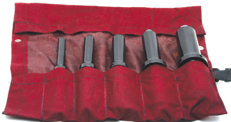
Combo Flare & Rerounding Tools in handy canvas carrying bag
